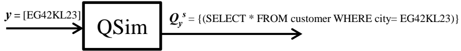
Fig. 4. QSim takes ciphertext query tokens as input and builds a set of rewritten SQL queries out of them.
